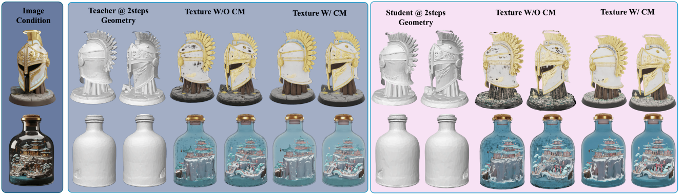
Figure 1: The few-step distribution shift and its correction by CM . From left: input image; the untextured mesh and PBR render of our two-step student without Channel Match, where the sampling-induced shifted shape latent drives the frozen PBR texture model to produce faulty surface materials (dark/blotchy patches); and the mesh and render with CM . For both few-step teacher and student sampling, calibrating the latent removes the texture artifacts, while the geometry remains unchanged. (We consider samples with simple geometry here, where both the two-step teacher and our two-step student already recover structures close to the many-step reference. This controlled setting isolates the effect of latent distribution shift rather than geometry reconstruction errors, showing that the shift is a general issue of few-step sampling and can be effectively corrected by CM .)
